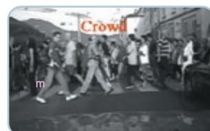
*Continuous tracking of pedestrians even when temporarily occluded by pedestrians walking in opposite directions. Crossing pedestrians marked in red and static in white.*
