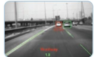
The headway value equals the distance to the vehicle ahead divided by the driving speed.
