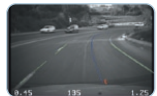
Lane detection and road geometry estimation on a winding road
