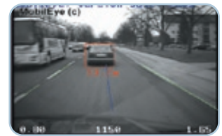
Urban LDW - detection of curbs when no lane markings exists
