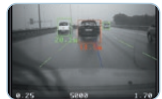
Lane detection in heavy rain
